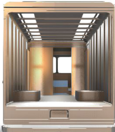
Twin Skylight Roof
